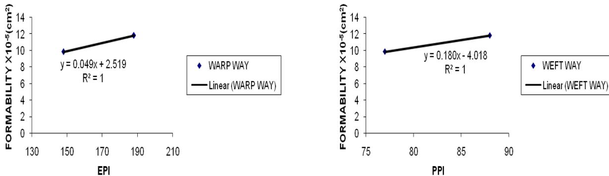
Figure 4. Effect of Fabric Weave Density on Formability with warp way and weft way (for plied yarn)
