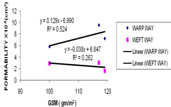
Figure1. Effect of GSM on Formability from warp way and weft way
