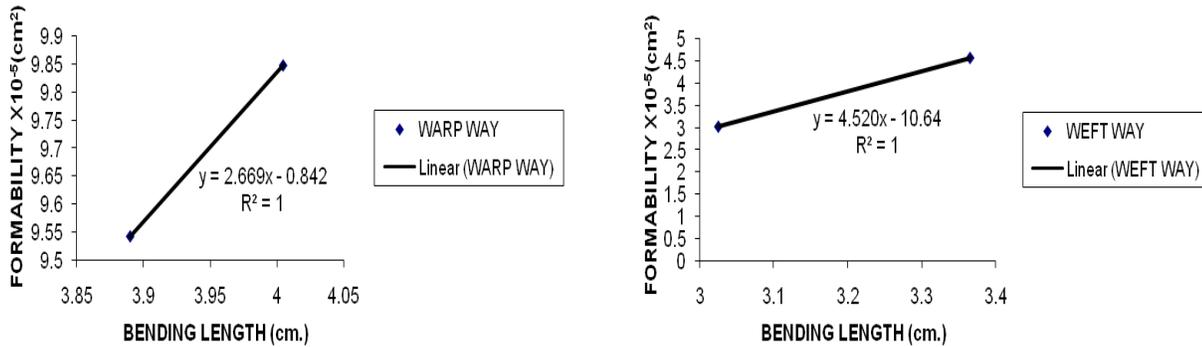
Figure 3. Effect of Bending Length on Formability with warp way and weft way
