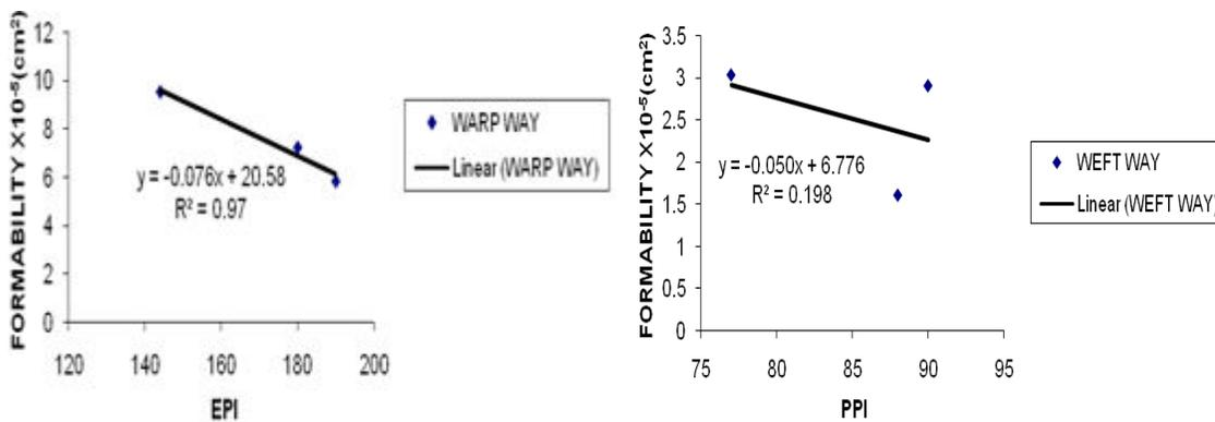
Figure 5. Effect of Fabric Weave Density on Formability with warp way and weft way (for single yarn)
